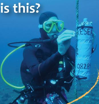
An **ACOUSTIC RECEIVER** is a listening station that 'hears' the unique pings from a fish tagged with an **ACOUSTIC TAG**.
